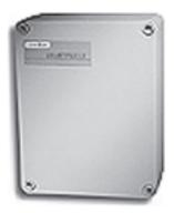
The Cardax SmartProx Long Range is a long range card only proximity reader. It has a read range of up to 2 metres depending upon the transponder type. The antenna is a simple wire loop which can be built into the surrounding structure.
